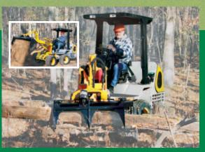
New multi-purpose SuperBee converts to a loader in about 45-minutes with bolt-on bucket and lift arms.
