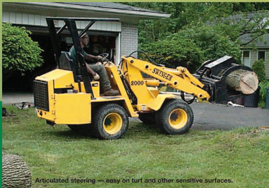
Swinger Model 2000 has 65 hp Cummins diesel.
