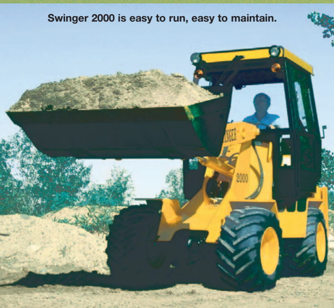
Swinger Model 2000 has 65 hp Cummins diesel.
